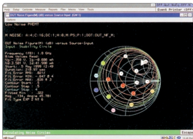
Example plot of noise figure versus the source states presented by the input tuner to a low-noise PHEMT. Note the full spread across the Smith chart and noise circles.
